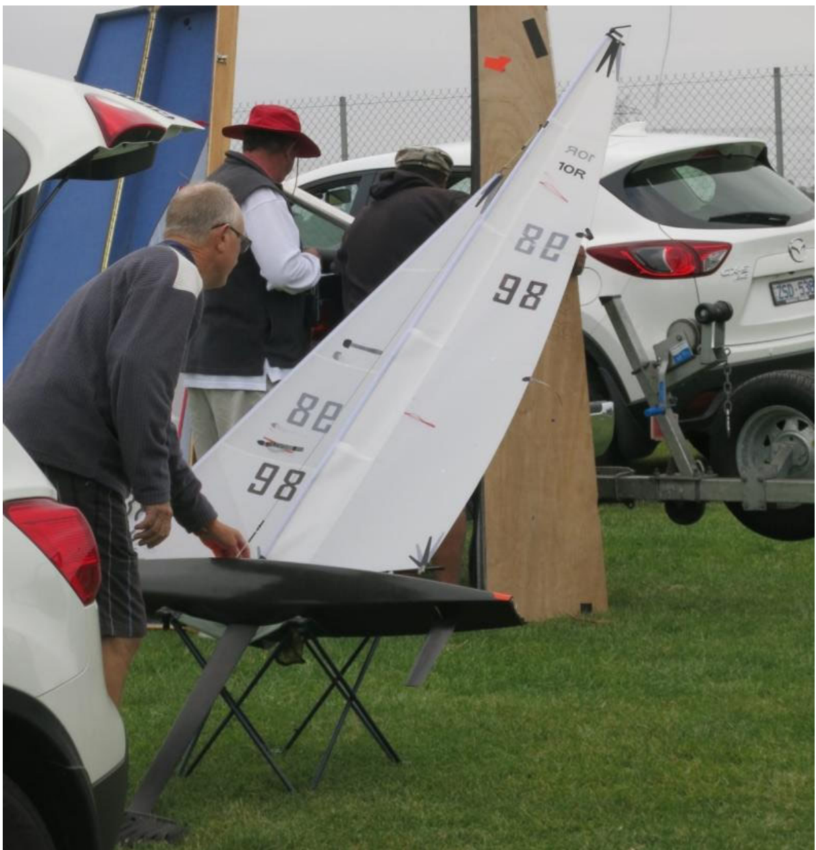
Selwyn Holland with his Aero 3 and a suit of Sedmen sails, using the wrap around mainsail constructed with a single sheet of material behind the pocket
