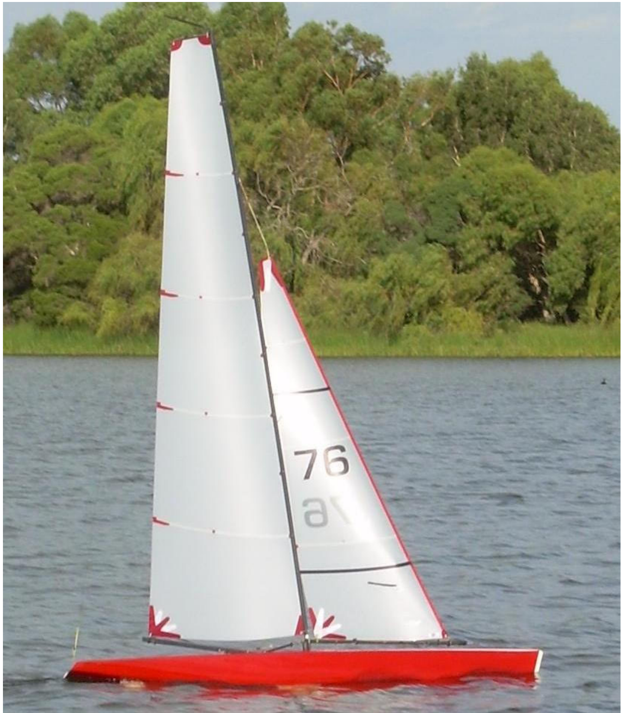
Glenn Dawson's Blade with the experimental square top mainsail
