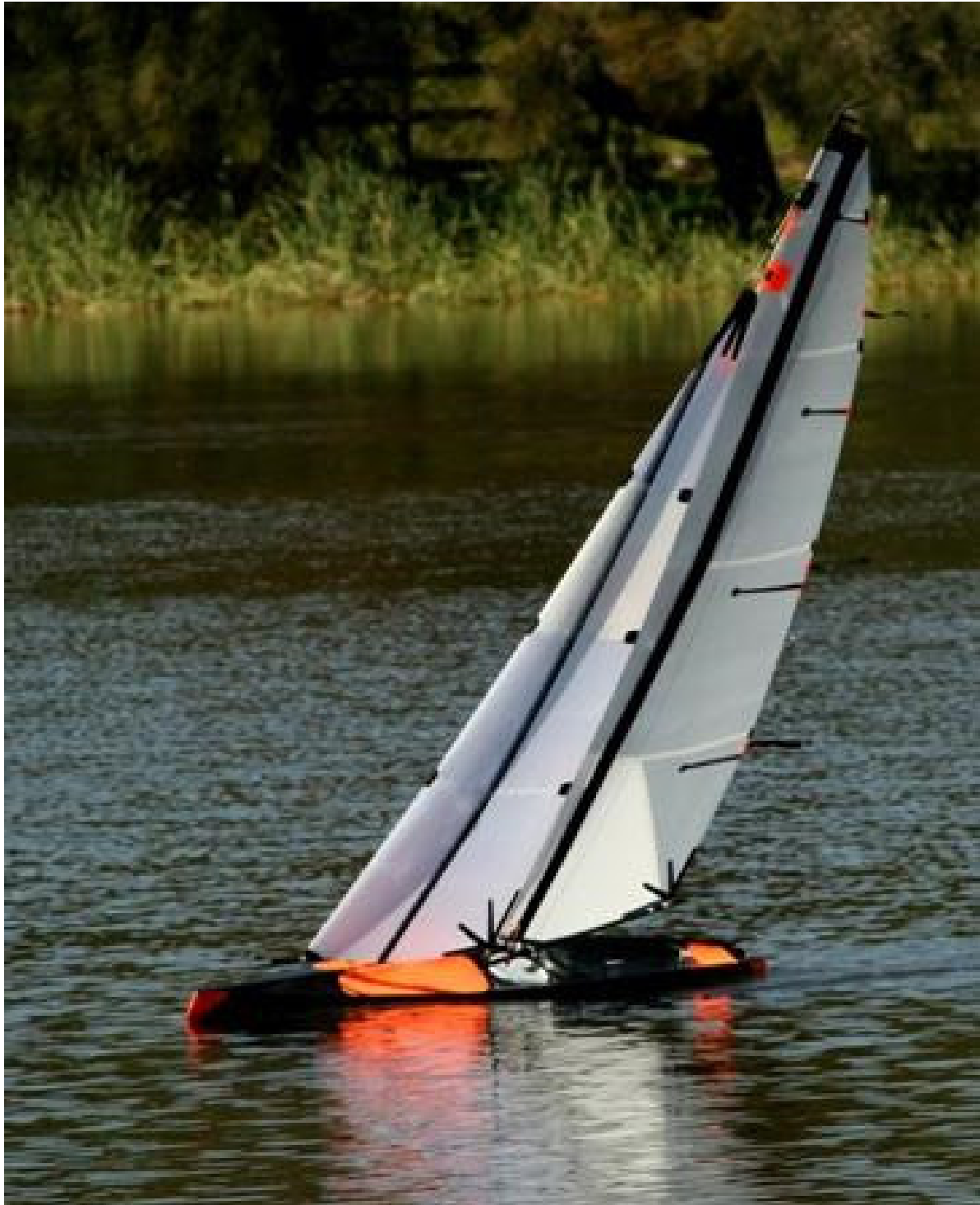
An early image of Selwyn's first prototype with the wrap around jib.
