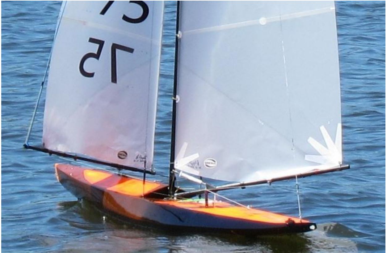
Offbeat again. The bow-up attitude indicates it needs more weight in the bulb, but I am reluctant to get the scissors out just yet
