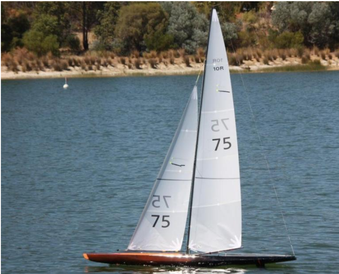
My own design, Offbeat, built over a plug whilst my wife was out of the country! An exercise in massive overhangs – it's 181cm long!
