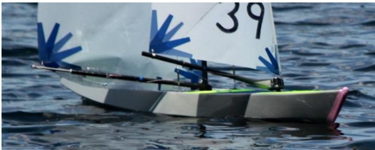
The radial jib fitting that was installed 6 months later
