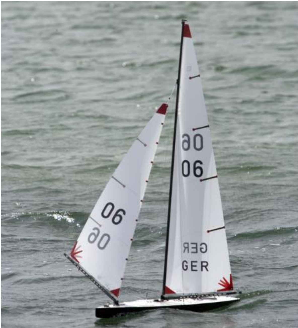
A Partner running downwind, with the radial boom goosewinged by the butterfly fitting located on the hull just in front of the mast
