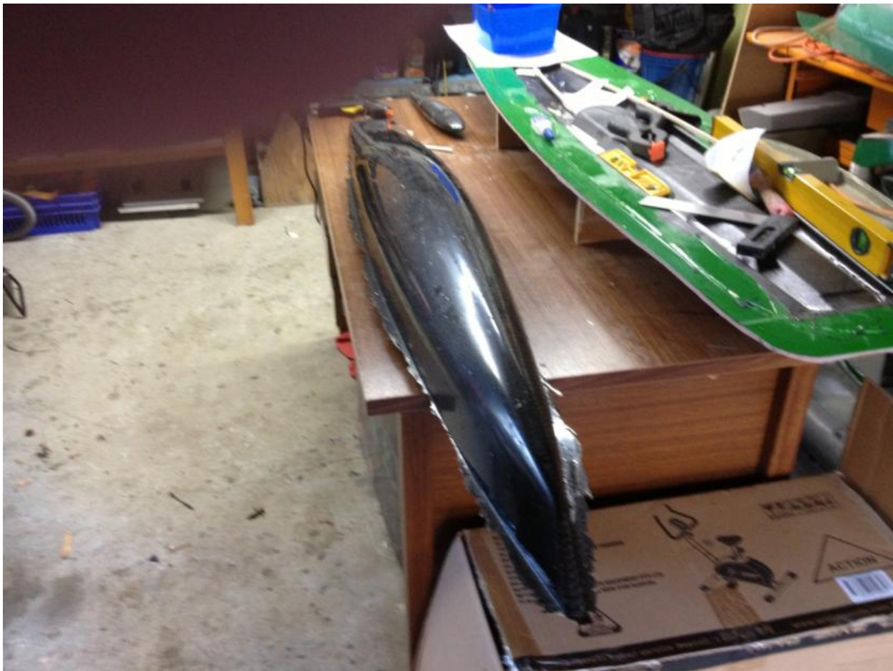
Raptor V: Not easy to see but there is a flat forefoot to the bow
